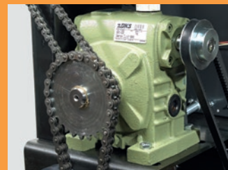
Full Size Gearbox Heavy-duty 30:1 ratio gearbox
