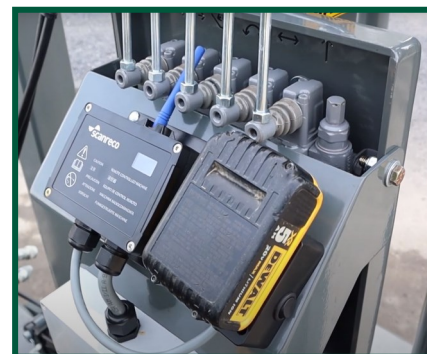
Remote Control Hydraulic Upgrade Scanreco electronics powered by DEWALT or MILWAUKEE battery.
